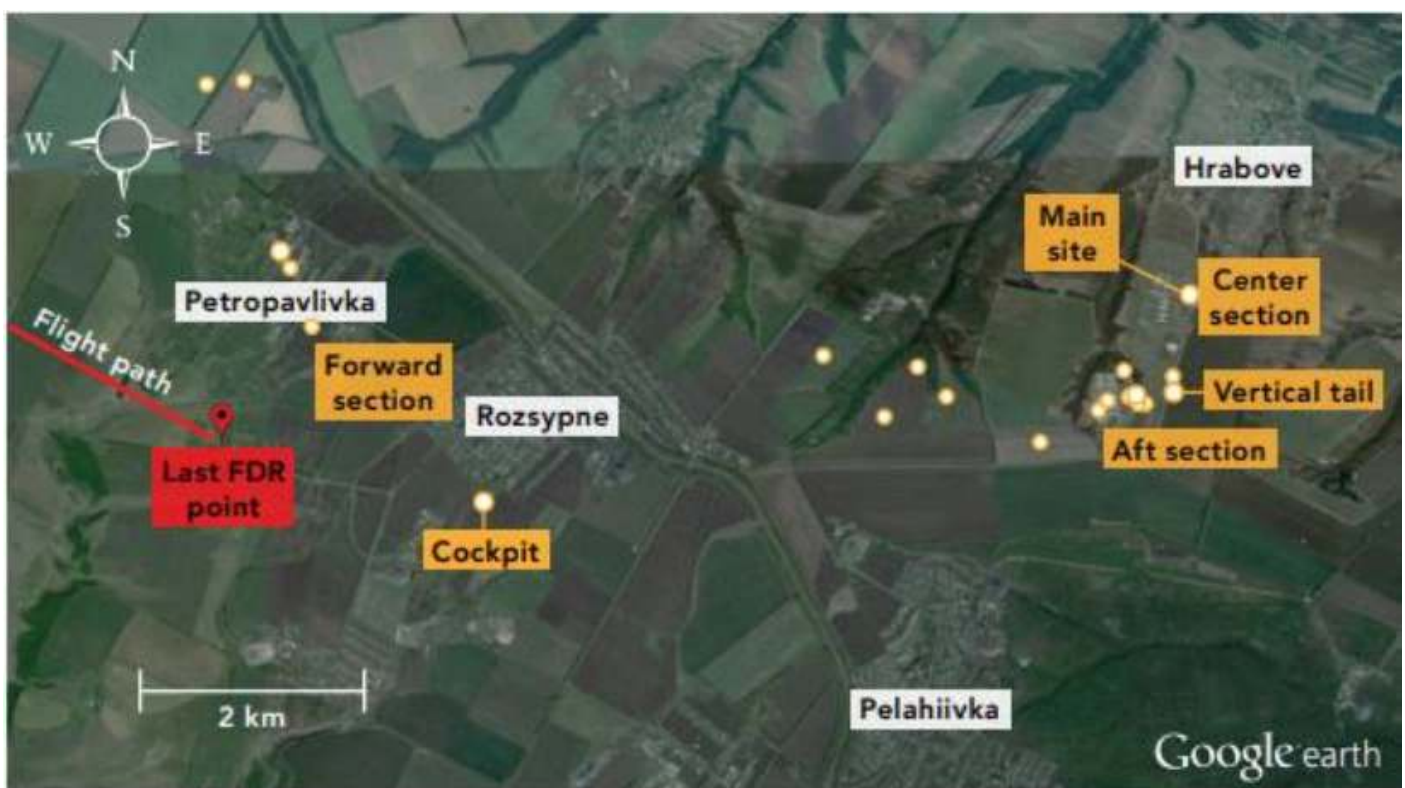
Figure 6: The last location of the aircraft in flight taken from the FDR. Wreckage distribution is grouped per section of the aircraft (Source: Google Earth, wreckage information Dutch Safety Board).
